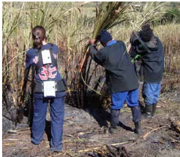
Figure 2: Tester fitted with the Lumbar Motion Monitor in order to assess spinal kinematics of the sorting task.
